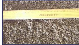
A washed sand that has 100% passing the 3/8" sieve. Used for ready mix applications and may be used in other applications.
