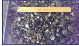
A 1" aggregate that has 100% passing the 1 1/2" sieve with 95-100% passing the 1" sieve. Typically used as a concrete aggregate and may be used in other applications. Sometimes referred to as #57 aggregate.
