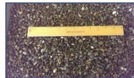
A 3/8" crushed aggregate which must have 100% passing the 1/2" sieve and may have material retained on the 3/8" sieve.
