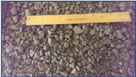
A crushed permeable material used for drainage applications and may be used in other applications.
