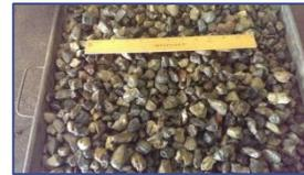
A 3/4" crushed aggregate which must have 100% passing the 1" sieve and may have material retained on the 3/4" sieve.
