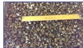
A 1/2" crushed aggregate which must have 100% passing the 3/4" sieve and may have material retained on the 1/2" sieve.
