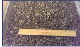
A 3/8" aggregate that has 100% passing the 1/2" sieve with 85-100% passing the 3/8" sieve. Typically used as a concrete aggregate and may be used in other applications.
