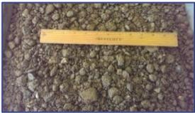
A permeable material used for drainage applications and may be used in other applications. Conforms to the specifications of Caltrans Section 68 (State of California, n.d.).
