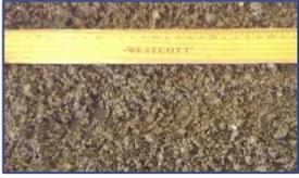
A sand-like material that has 100% passing the 3/8" sieve and may be produced using crushed fine materials. Typically an asphalt aggregate but can also be used in concrete and may be used in other applications.
