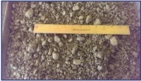
A 3/4" Class II aggregate base using only natural materials. Used in roadways as a base course in pavements and may be used in other applications.
