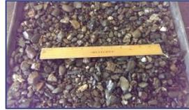
A 3/4" aggregate that has 100% passing the 1" sieve with 95-100% passing the 3/4" sieve. Typically used as a concrete aggregate and may be used in other applications. Sometimes referred to as #67 aggregate.
