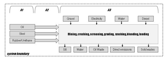
Figure 2. Main Processes Included in System Boundary
